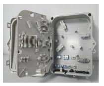
CISFIBER Infra Solution's Optical Termination Box (OTB) is FTTx box which is used to patch up to 24 fibers and splice up to 32 fibers. It can handle SCPC/SCAPC/LCPC/LCAPC/FCPC/FCAPC adaptors and connectors. This is a ruggedized termination box with IP65 compliant rating.
